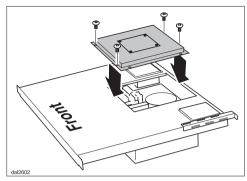
■ When finished, mount the previously removed cover on the front.
